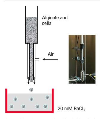
**Figure 2. Schematic representation of the air-driven droplet generator.** The figure depicts the principle of encapsulation (left) and the encapsulation apparatus (right) attached to a 1 ml syringe containing the cells and alginate suspension.
